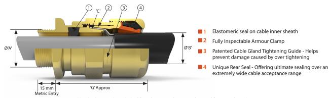
The 153/RAC Cable Gland is an industrial gland for indoor or outdoor use, robust and for use with single wire armour 'W', wire braid 'X', steel tape armour 'Z', elastomer and plastic insulated cables. The gland provides an elastomeric seal on the cable inner sheath, and a low smoke, zero halogen IP and retention seal onto the cable outer sheath.
